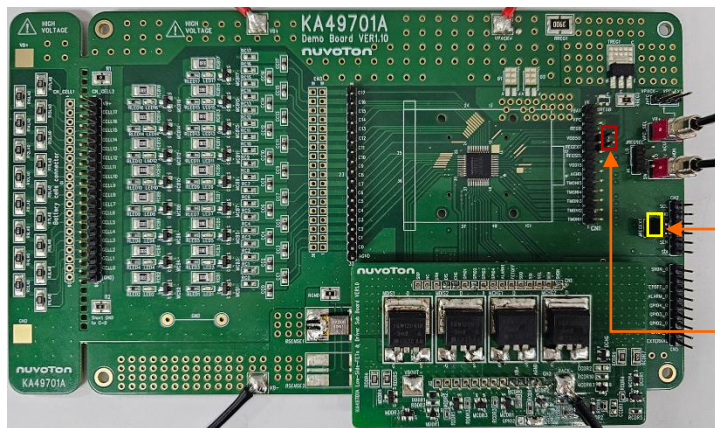
Figure 3.3 REGEXT supplies to MCU controller board.
