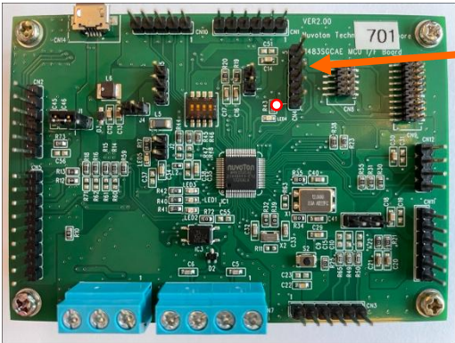
Figure 2.7 Serial Wire Debug (SWD) Interface connector (CN4)
